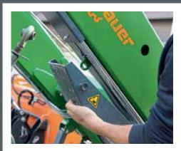
Folded into storage position, the parking stands automatically cover the pipework offering excellent protection should the boom foul with trailer sides.
