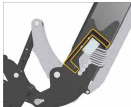
The steel sections have five edges and the cross beam is double-walled, providing a torsion-free structure that withstands the toughest conditions. The cross beam is mounted at an angle to adopt the operator's line of vision for best visibility.
